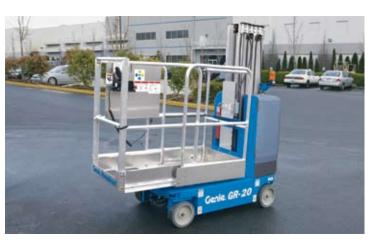
**SLIDING MID-RAIL EXTENSION DECK PLATFORM** 55 x 29.5 in (140 x 75 cm) Provides 20 in (51 cm) of horizontal outreach and a larger work area within the platform.
